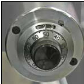
A micrometer style digital readout makes crimp set up easy and precise
