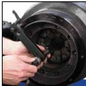
A coupling stop and a retraction stop makes production crimping a fast and repeatable process.
